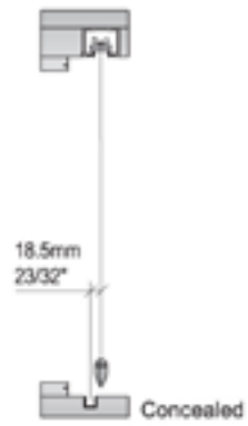
Figure 36: Front alignment measurement offset
