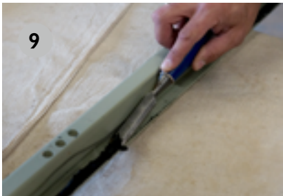
Whilst most of the bonding tape should be removable by hand it may be necessary to use a blunt tool to carefully remove the tape, being careful not to damage the paintwork.
