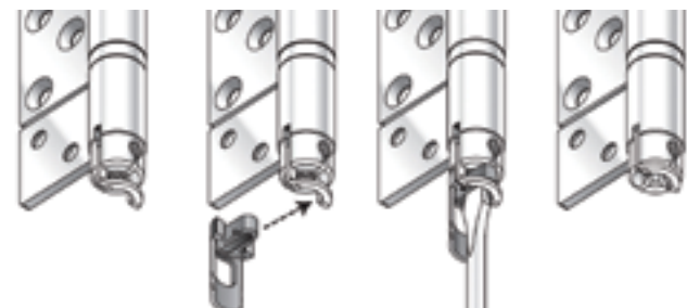
Figure 39: Vertical adjustment with shipping clip
