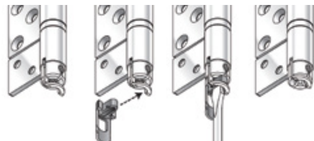
Figure 38: Vertical adjustment with shipping clip
