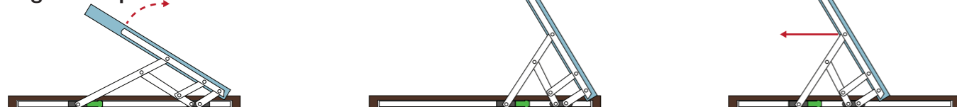
Figure 02: Operation of restrictor and easy clean hinges
